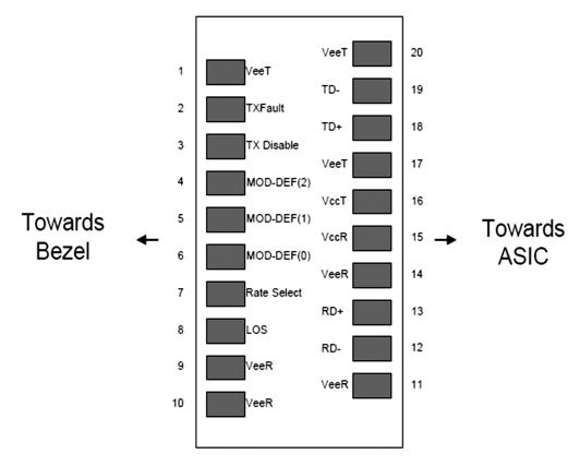
Pinout of Connector Block on Host Board
